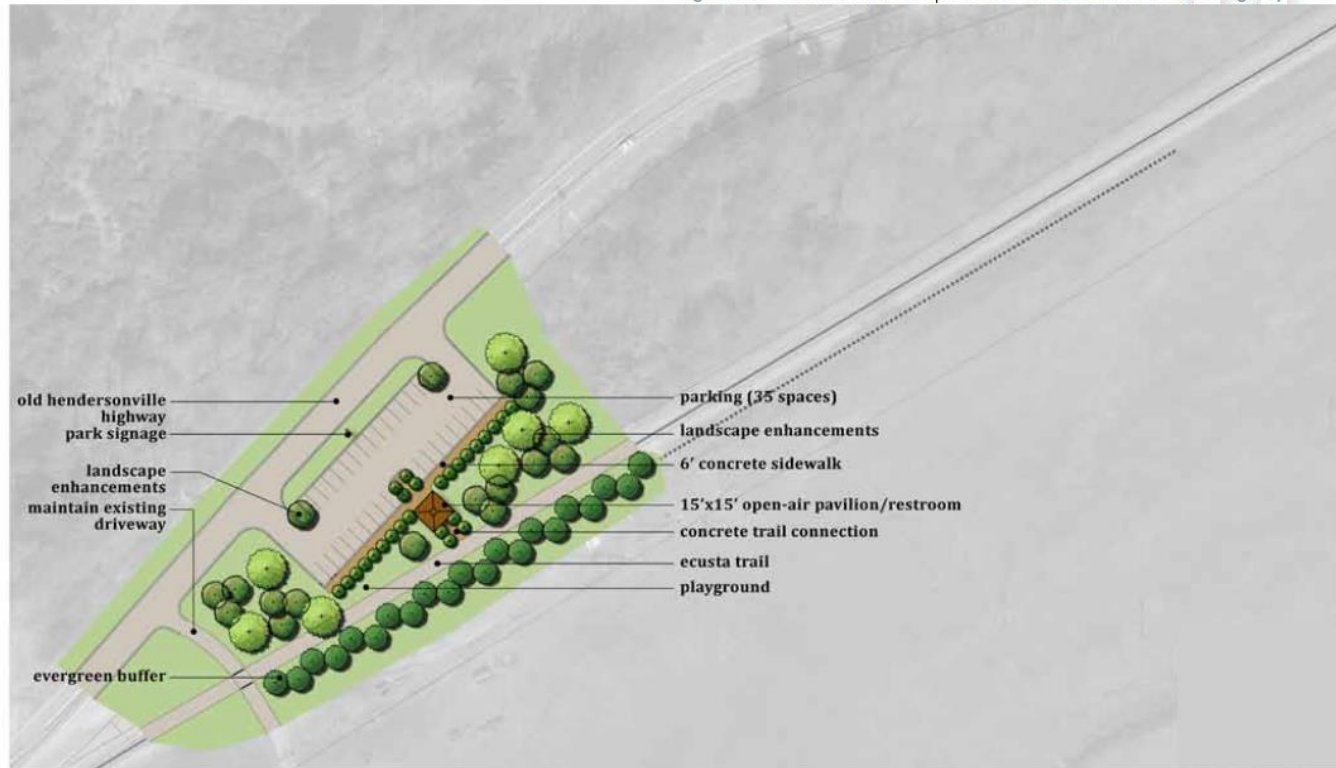
Figure 6.19— Potential Trailhead at Everett Road & Old Hendersonville Highway
