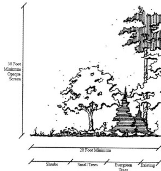
FIGURE 8.4C: TYPE D BUFFER YARD
