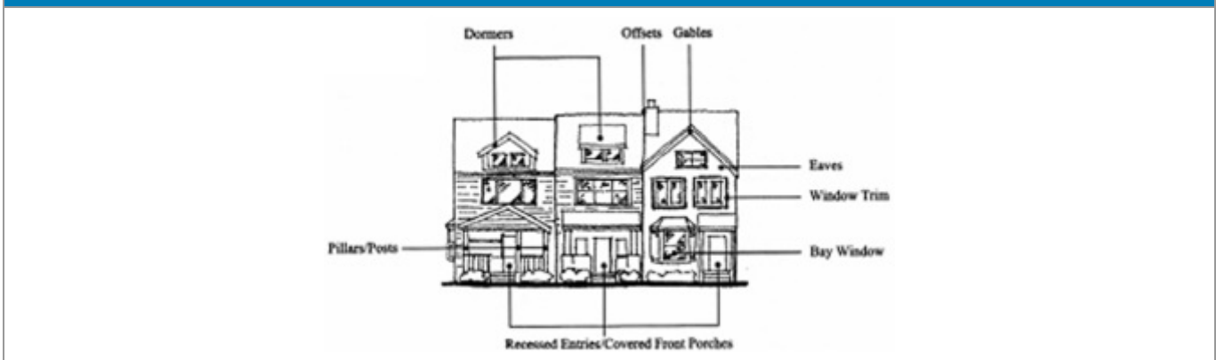
FIGURE 5.11C : ILLUSTRATION OF TOWNHOUSE BUILDING FACADE
