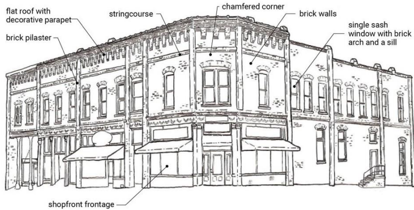
FIGURE 5.8.1-A: BRICK MASONRY VERNACULAR ILLUSTRATIONS
