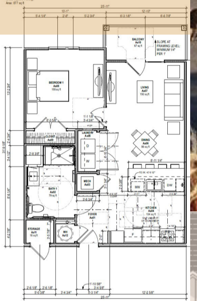
Unit A(a)1 - Type A 1 Bedroom / 1 Bathroom Accessible w/ Roll-In Shower Net Square Footage: 732 sq ft Gross Square Footage: 877 sq ft
